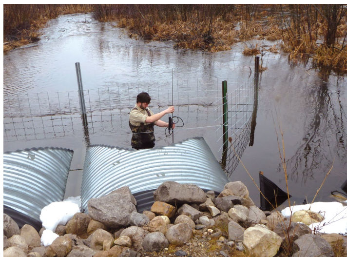
Lab technician Blaze Budd measures discharge using an OTT acoustic digital current meter at Black Creek within the Manistee River watershed.
