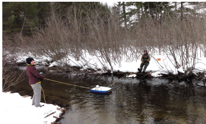
Undergrad student Brianna Jansinski and lab technician Blaze Budd perform a discharge measurement using a Sontek S5 acoustic Doppler current profiler on the East Branch Au Sable River.
